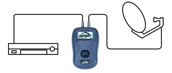
The **EZ-SAT** uses the receiver LNB power as illustrated above or utilizes an external battery pack accessory as shown below. The standard kit includes the following items.
